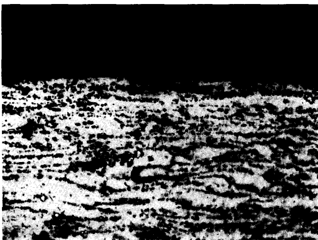
Fig. 6. Corrosion of wrought Pb-6wt.%Sb alloy. Magnification 200 \times .
