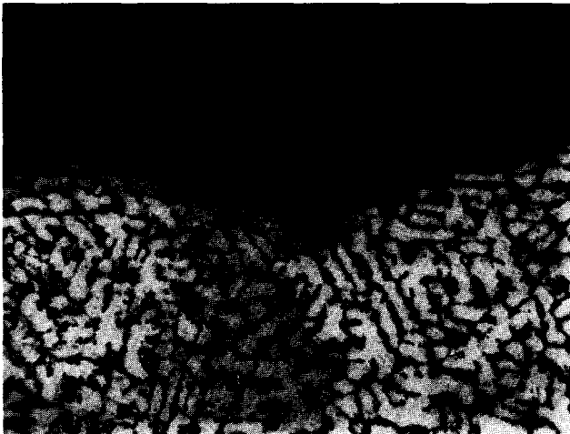
Fig. 5. Corrosion of cast Pb-6wt.%Sb alloy. Magnification 200 \times .
